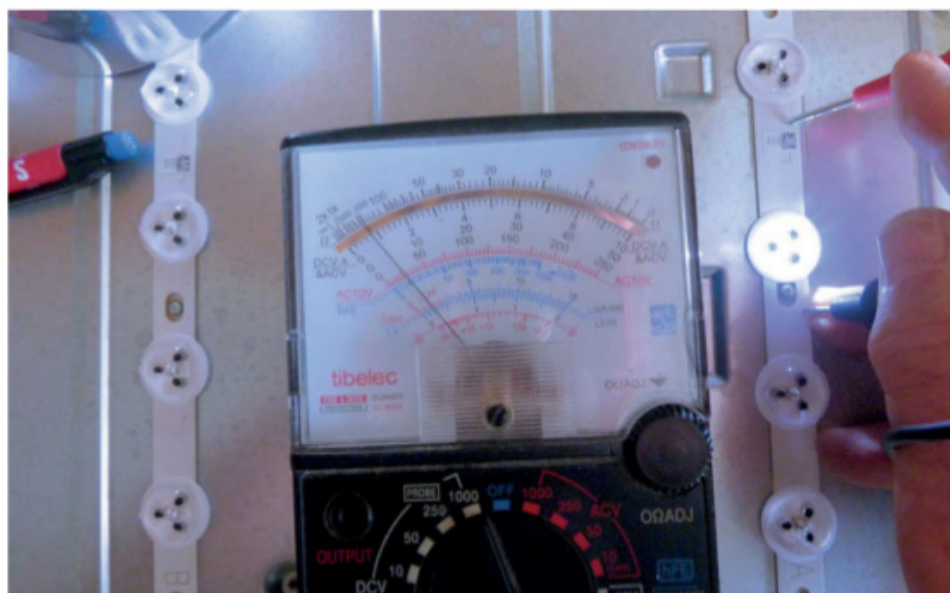
Figure 9-54. Test individuel des LED
