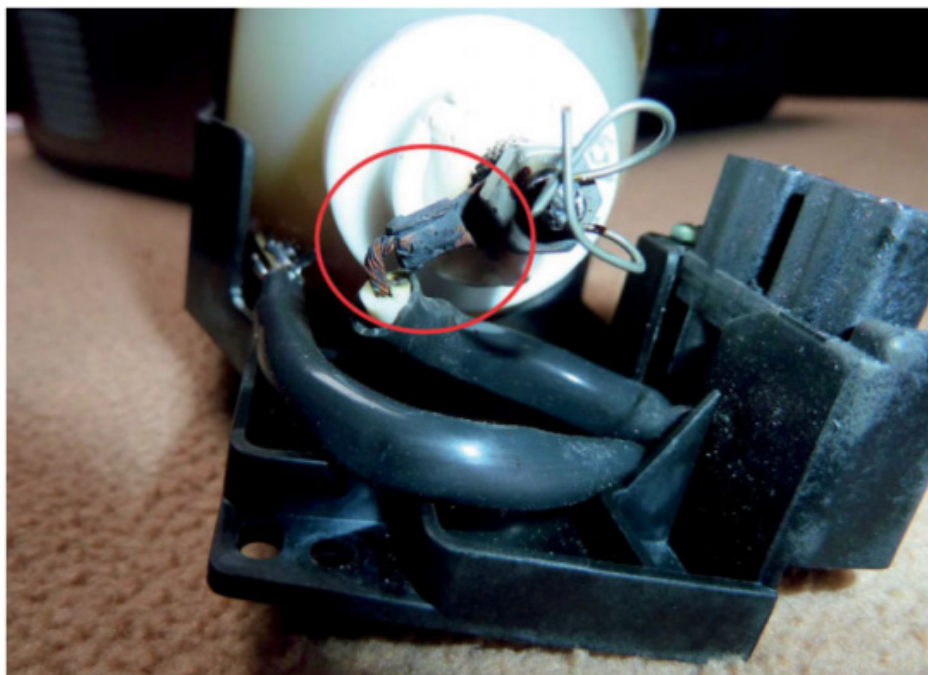
Figure 8-34. Connexion de lampe ayant surchauffé
